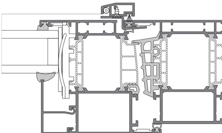
Horizontal cross-section - opening mosquito net
