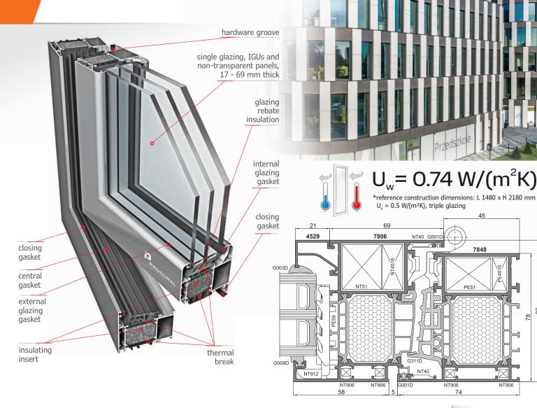
An insulated, three-cavity profile system designed for the construction of windows with very high thermal insulation requirements
