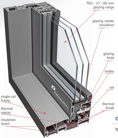
U<sub>w</sub> = 0.88 W/(m<sup>2</sup>K) \*reference construction dimensions: L 2400 x H 2400 mm A sliding system with insulated profiles designed for the construction of external joinery.
