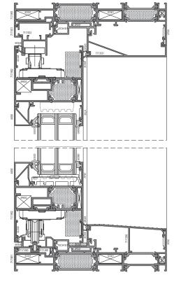
$U_q = 0.5 \text{ W/(m}^2\text{K)}$ , triple glazing
